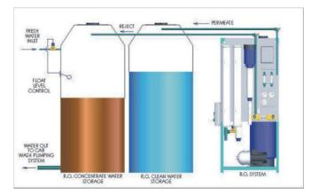
Typical Installation of the Storage and Repressurization Systems installed with RO in Carwash Application
