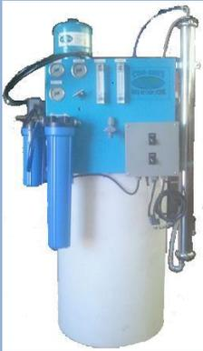
The **CSARO System** was designed to meet low flow applications in a minimal space. Permeate water is dispensed from a hose bib on the front panel via a Self priming pump. The Ro system replenishes the 65 Gallon storage tank automatically. On/Off operation is controlled by level controls in the tank
